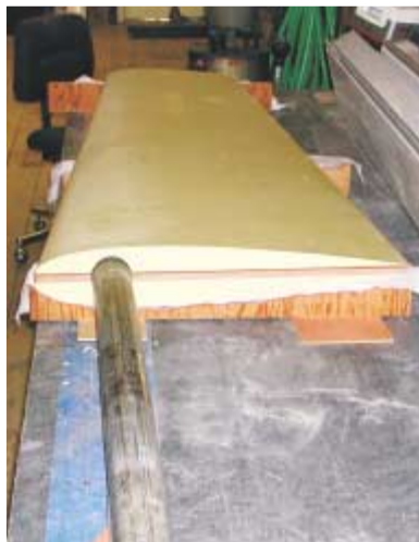
Right—The two foam halves, with the plywood core, are dry fit around the post before bonding.
