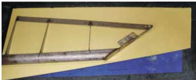
Above—The outline of the post and weldments were traced onto half of the foam. A router with a ¼" straight bit quickly removed the foam.
